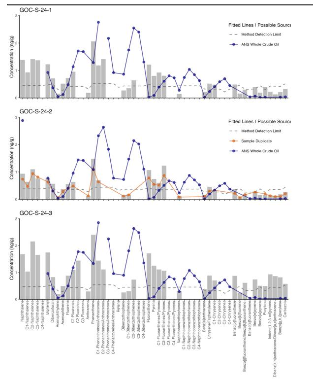
**Figure 3.** 2024 PAH profiles from individual sediment samples at the Gold Creek (GOC) reference site with the ANS potential source profile, sample duplicate, the analyte-specific method detection limit superimposed as different lines. ANS profile lines are scaled to Napthobenzothiophenes in the third replicate and represent data only where points are present.
