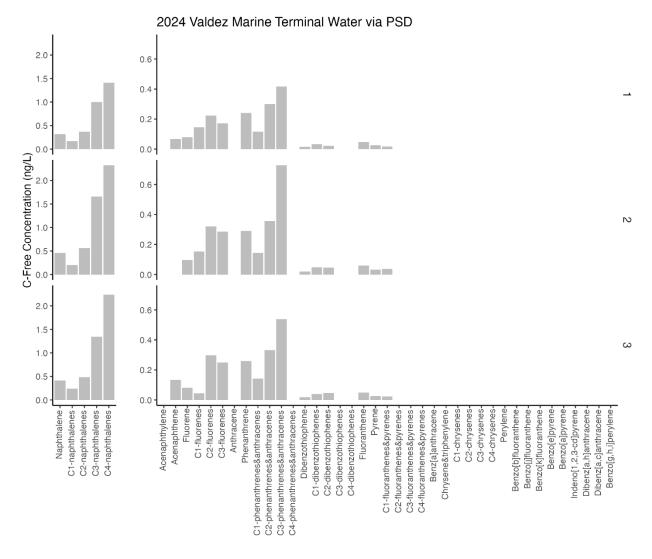
**Figure 22.** PAH profiles in seawater sampled via passive sampling devices placed at Valdez Marine Terminal in 2024. Values represent the reported values for the three replicates stacked vertically. Note the changes in scale between the Naphthalenes on the left and the other PAHs.
