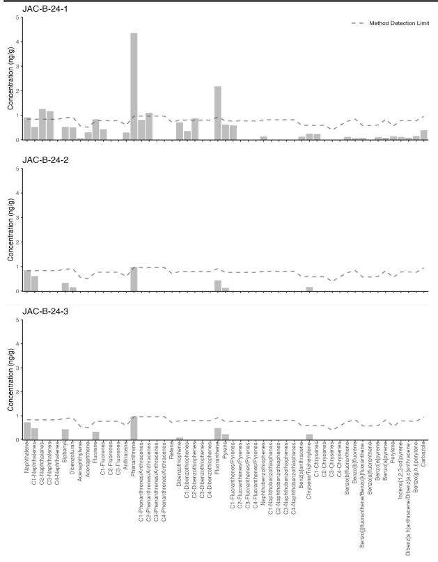
**Figure 9.** 2024 PAH profiles from individual tissue samples at the Jackson Point (JAC) site, near the Valdez Marine Terminal, with the analyte-specific method detection limit superimposed as a dotted line.
