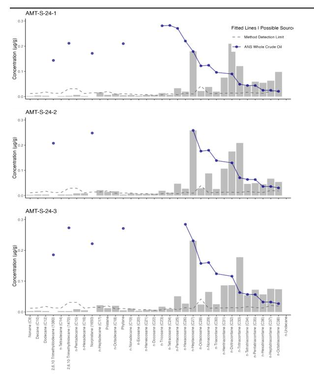
**Figure 6.** 2024 saturated hydrocarbon profiles from individual sediment samples at the Valdez Marine Terminal (AMT) with the ANS potential source profile and the analyte-specific method detection limit superimposed as different lines. ANS profile lines are scaled to n-Heptacosane (C27) and represent data only where points are present.
