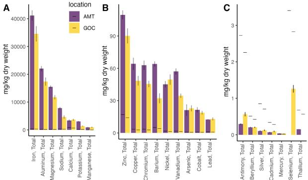
Figure 2. Sediment metal concentrations are displayed as a bar plot with mean ± standard deviation for Valdez Marine Terminal (AMT) in purple and Gold Creek (GOC) in yellow. Dashes represent the mean metal-specific reporting limit. Note that each panel has a different scale.
