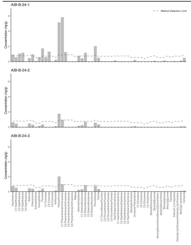
**Figure 12.** 2024 PAH profiles from individual tissue samples at the Aialik Bay (AIB) site, near the Valdez Marine Terminal, with the analyte specific method detection limit superimposed as a dotted line.
