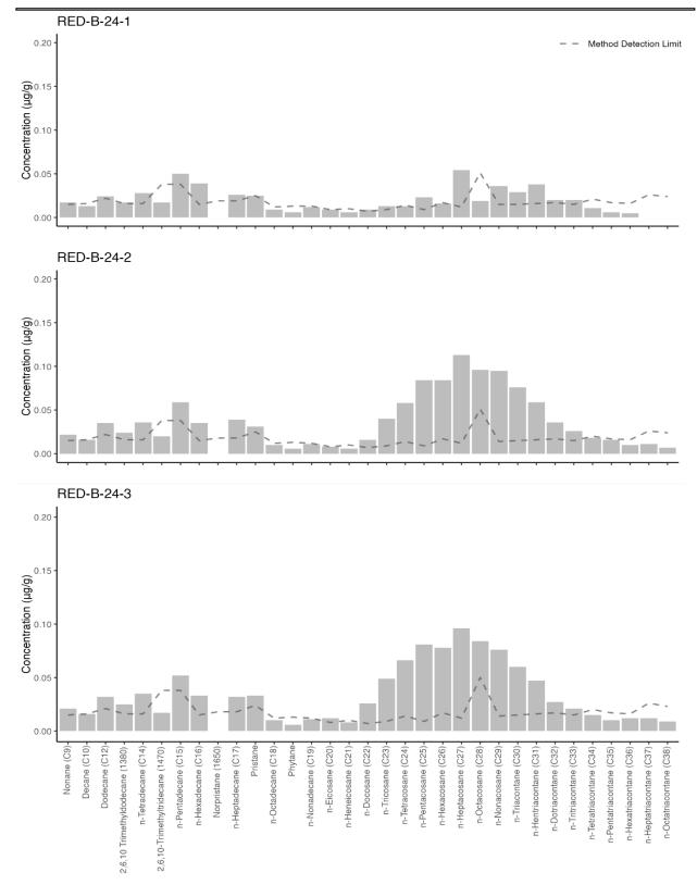
**Figure 18.** 2024 saturated hydrocarbon profiles from individual tissue samples at the entrance of the Valdez Small Boat Harbor (RED) site with the analyte-specific method detection limit superimposed as a dotted line.
