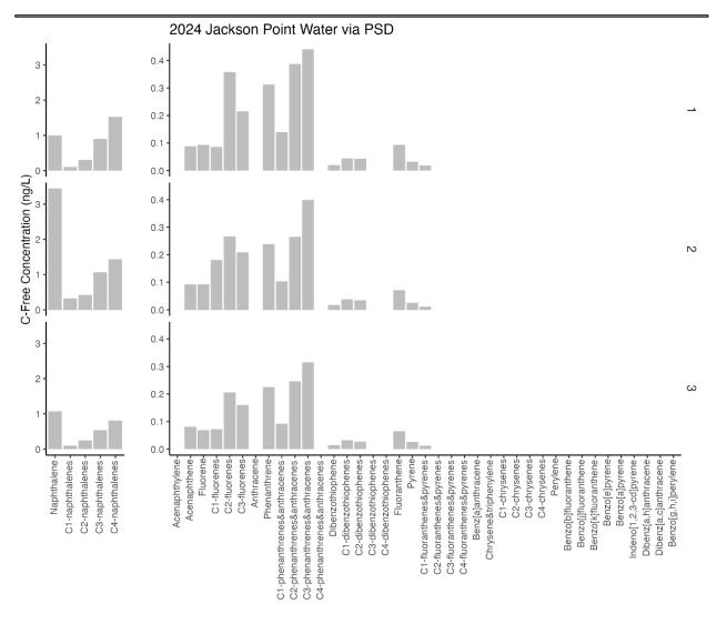
**Figure 23.** PAH profiles in seawater sampled via passive sampling devices placed at Jackson Point in 2024. Values represent the reported values for the three replicates stacked vertically. Note the changes in scale between the Naphthalenes on the left and the other PAHs.
