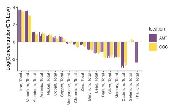
Figure 3. Sediment metal concentrations normalized to the Effect Range Low (ERL) value, shown on a log scale and organized by the degree of ERL threshold exceedance. Each sample replicate is displayed individually. Bar colors represent location. Metals that do not surpass the ERL threshold have negative values due to the log scale. Metals without an ERL threshold are excluded from the plot.
