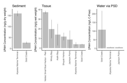
Figure 2. Sum PAH concentrations for 2024 sediments, Pacific blue mussel tissues, and water sampled via passive sampling devices by site plotted at the mean ± 1 standard deviation. Note the unit difference between matrices (i.e., parts per billion for sediments and mussel tissues, and parts per trillion for passive sampling devices).
