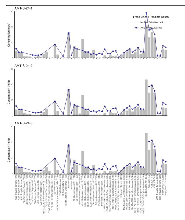
**Figure 4.** 2024 petro-geochemical profiles from individual sediment samples at the Valdez Marine Terminal (AMT) with the ANS potential source profile and the analyte-specific method detection limit superimposed as different lines. ANS profile lines are scaled to Hopane (T19) and represent data only where points are present.
